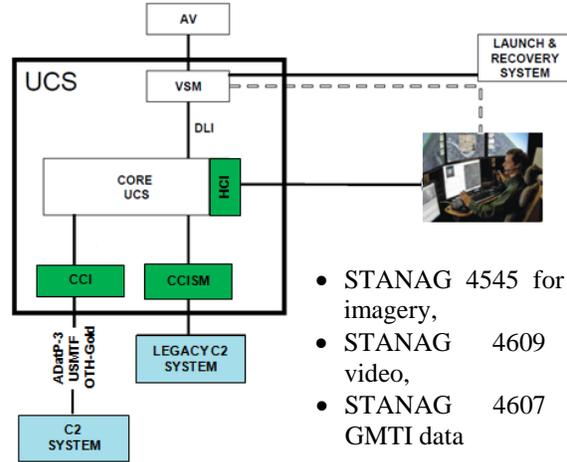
Figure 2 – UCS Interface Functional Architecture
