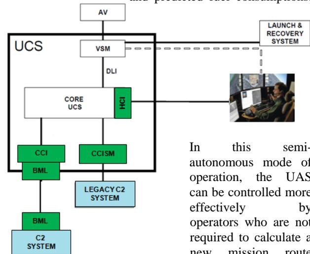
Figure 4: BML-Equipped UAV UCS
